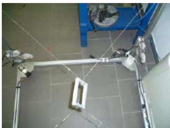
Figure 6 The CALOWI (Cassino Low-Cost Wire System) robotic system.
