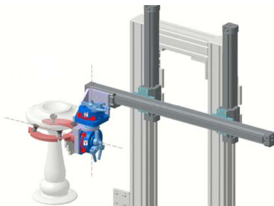
Figure 12 Movements character of rotary actuators in different axes.
