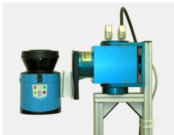
Figure 7 Tilting laser range scanner for capturing the test data.
