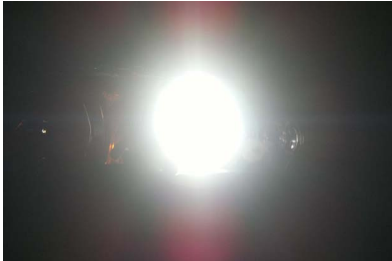
Figure 17: Headlight with xenon no-filters lamp, with a hidden by backlighting object.
