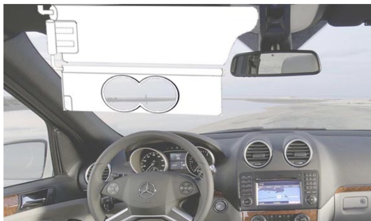
Figure 3 Internal polarizer screen installed on a foldable support in the sun visor set.chart.
