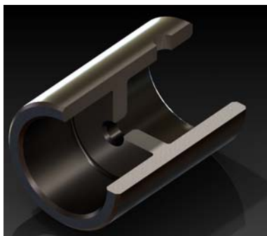
Figure 2 Sectional view of the sleeve.
