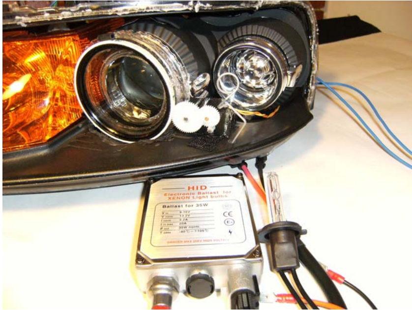
Figure 10: Xenon lamp with its power supply, before being inserted in the parable
