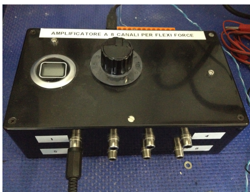
Figure 2 The amplifier based on the suggested op-amp drive circuit.
