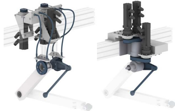
Figure 10 Concepts G (left) and I for the actuation of the arm.
