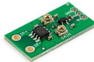
Figure 10 Customized module for servo current measurement (Sparkfun 2012).
