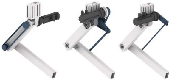
Figure 6 (a-c) Combination of motor 3 at link 1 and transmission between A and B.
