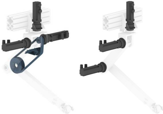
Figure 8 Concepts C (left) and D for the actuation of the arm.
