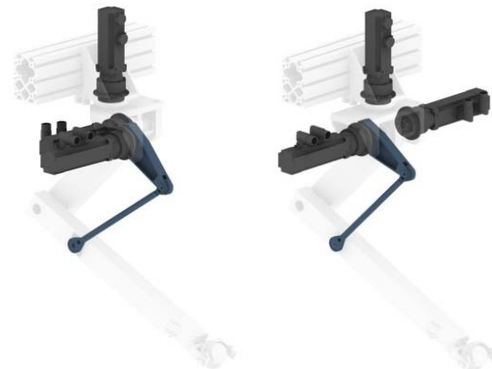
Figure 7 Concepts A (left) and B for the actuation of the arm.
