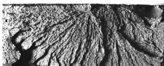
Figure 6 Radiating Ridge Fracture Surface [2].
