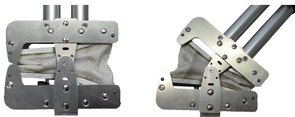
Figure 3 sREC actuator with skewed chambers (construction with unsymmetrical working range from 0 to approx. 45°).
