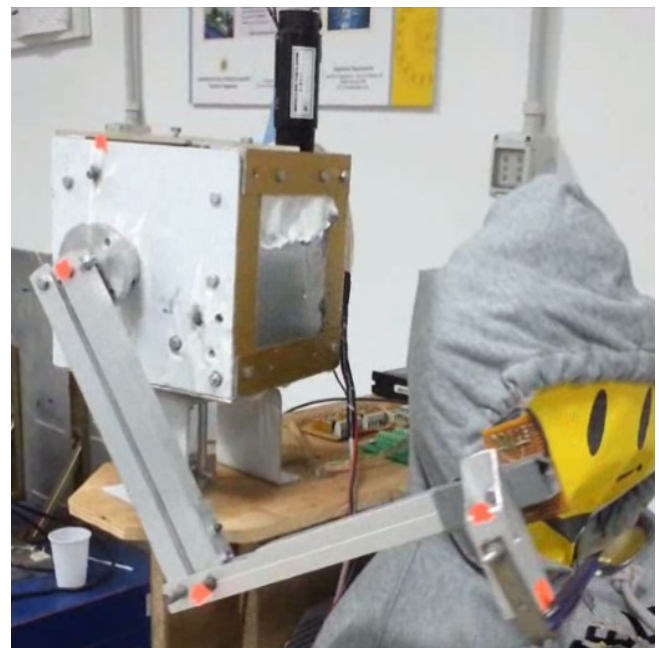
Figure 5 The prototype of LARM clutched arm in a lab setup for testing.
