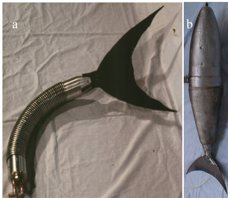
Figure 10 The actuator and fin integrated system and the fish like robot.
