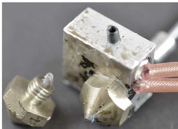
Figure 5. Example of clogged extruder.
