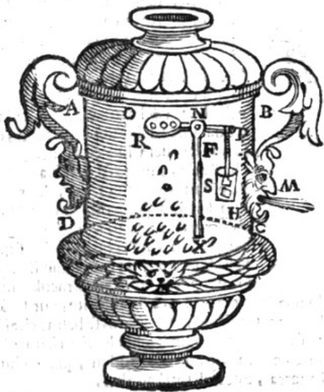
Figure 6 Aleotti's drawing of an Heron's vending machine.
