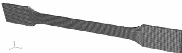
Figure 1 FE model (5852 eight-nodes brick elements).
