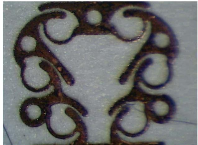
Figure 15 Prototype obtained by using copper electrodeposition.
