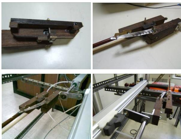
Figure 7 Details of the bow support.
