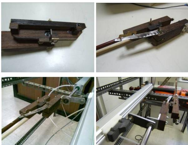
Figure 7 Details of the bow support.
