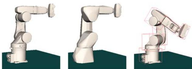
Figure 11 3D models for robot and laser probe: accurate (for rendering), convex and intermediate oriented boxes (for fast collision detection)
