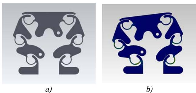
Figure 13 View of the 3D model with different way of wire attaching: a) unloaded structure; b) the structure under the effect of the applied load (treated with FEA).
