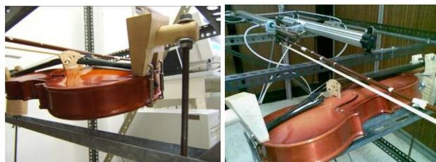
Figure 5 Connections between instrument and swivel-linear actuator.
