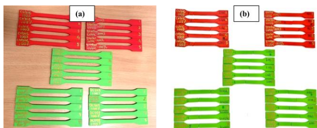
Figure 4 The samples with different infill pattern group after 3D printing (a) and after tensile testing (b).
