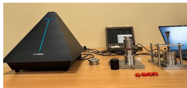
Figure 7 Experimental setup for thermal conductivity measurement of PLA sample printed with different infill geometries using the C-Therm Trident thermal analyser with MTPS sensor.
