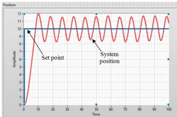
Figure 8 System behavior with proportional control (P) [15].
