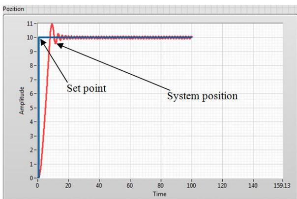
Figure 9 System behavior with proportional and integrative control (PI) [15].
