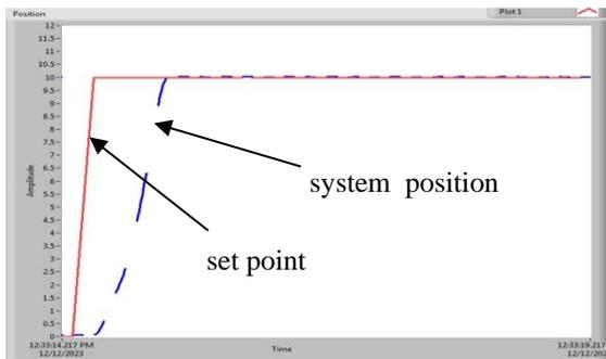
Figure 12 Experimental measurement of positioning.
