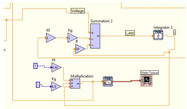
Figure 6 The program built for the simulation of the electric motor [15].
