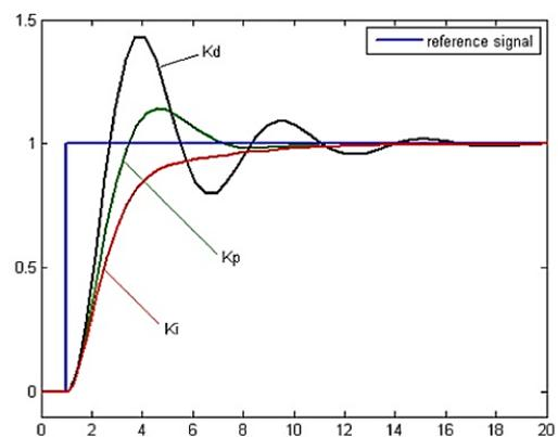
Figure 3 Effects of each of the controllers  $K_p$ ,  $K_D$ , and  $K_I$  on a closed-loop system [8].
