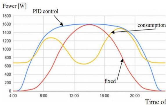
Figure 8 Blue line - the production of panel with PID control; Red - fixed mounted panel in roof; Yellow - family consumption
