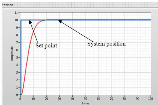
Figure 10 System behavior with PID control [15].
