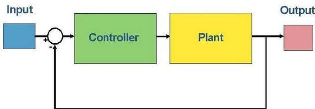
Figure 2a Closed Loop Control [9].
