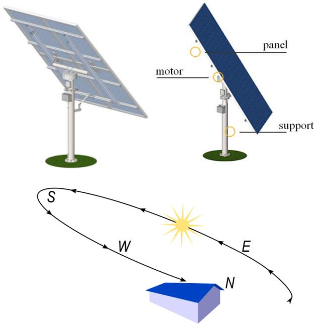
Figure 4 The trajectory of the sun's movement and the way the panel moves [9].
