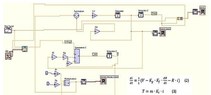
Figure 7 PIDcontrol built into LabView [15].
