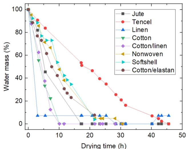
Figure 2 Water retention tests on different textile fabrics.
