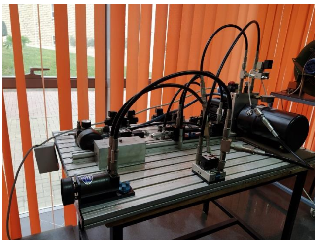
Figure 3 Experimental panel for measuring valve characteristics [15].
