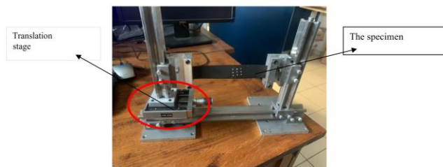
Figure 4 Loading machine production.
