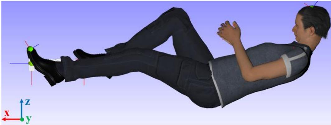
Figure 1 Lateral view of the 95<sup>th</sup> percentile male dummy with the global reference system (xyz).
