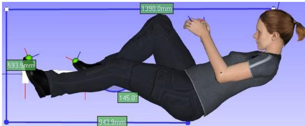
Figure 3 The 5<sup>th</sup> percentile female dummy with the encumbrance dimensions in the sagittal plane.
