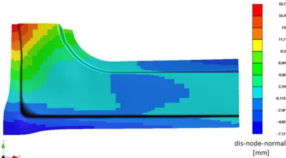
Figure 3 The displacements result after springback with extrapolation SHS law and friction coefficient 0.12
