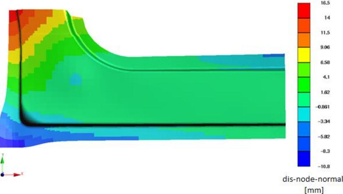
Figure 4 The displacements result after springback with extrapolation SHS law and friction coefficient 0.08
