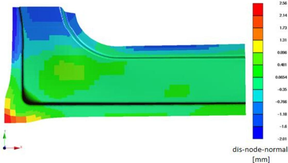
Figure 6 The relative displacements result with friction coefficient 0.16/0.08
