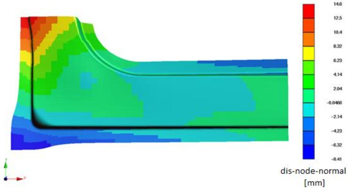
Figure. 5 The displacements result after springback with extrapolation SHS law and friction coefficient 0.16
