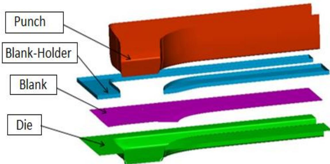
Figure 2. 3D view of the tools used for stamping.
