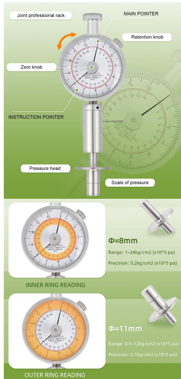
Figure 7 Images on top concern the joint professional rack and the main pointer of the device here utilized for penetrometer tests. Images below concern the two different reading scales of the pressure applied by the penetrometer on the sample to be tested depending on the diameter of each of the two usable pressure heads.
