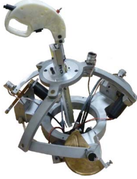
Figure 1 Master device of a tele-operation system.
