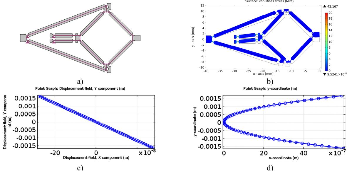
Figure 9 Compliant structures of modified Peaucellier-Lipkin mechanism a) mod\_02a; b) Stress and deformation of compliant Peaucellier-Lipkin mechanism (modification mod\_04c), Trajectory of output point of compliant PL SLM from FEM analysis c) linear solver, d) non-linear solver
