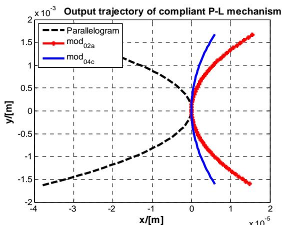
Figure 10 Output trajectories of modified compliant Peaucellier-Lipkin mechanisms compared with parallelogram
