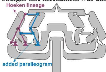
Figure 1 Structure of compliant micro-gripper with utilized Hoeken lineage for parallelly moving of fingers [10]
