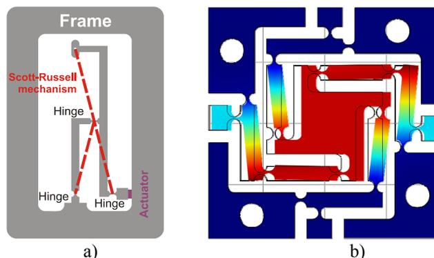
Figure 2 a) Nano-manipulation mechanisms based on Scott-Russell straight-line mechanism [12]; b) Design of our XY micro stage with minimized parasitic deformations based on Watt mechanism
