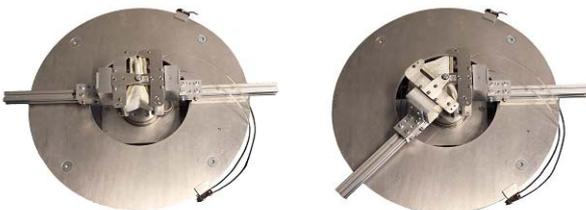
Figure 4 REC actuator mounted on the automated test-rig for torque characteristic measurements. The generated torque is measured at different angle-pressure combinations.
