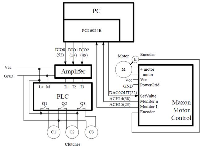
Figure 7 A block diagram of proposed control unit.
