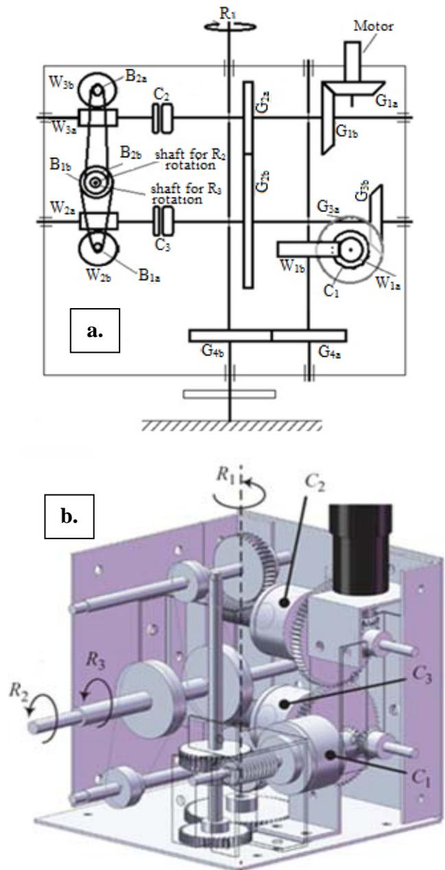
Figure 3 The mechanical shoulder design of LARM clutched arm; a) a kinematic scheme, b) a CAD model.
