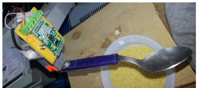
Figure 8 The accelerometer used at arm end point.
