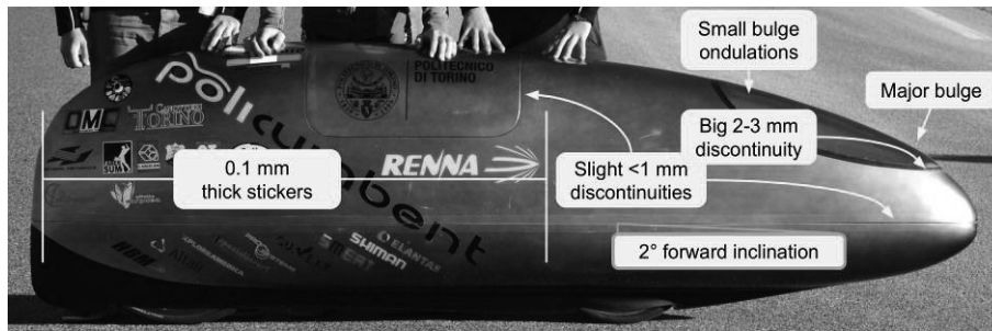
Figure 2 Pulsar 2015 with highlighted turbulent transition sources.
